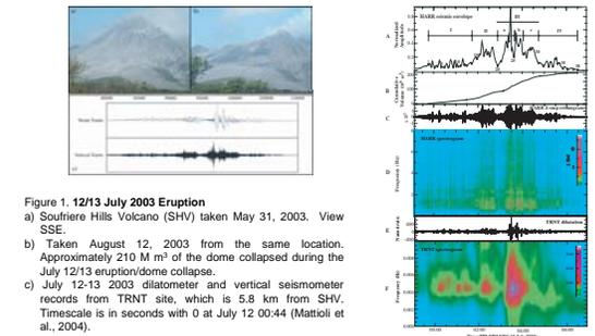
**Figure 5. Eruption Seismicity and Dilatation.**
