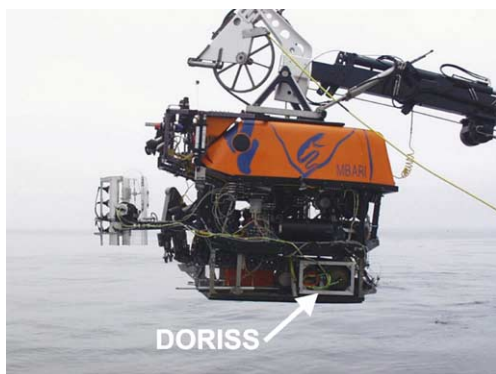
Fig. 2. The DORISS instrument on the ROV Ventana. The spectrometer housing and electronics housings are mounted in a drawer in the ROV tool sled (shown by arrow). The probe head is carried in front (left in the picture below) for deployment by the ROV manipulator.
