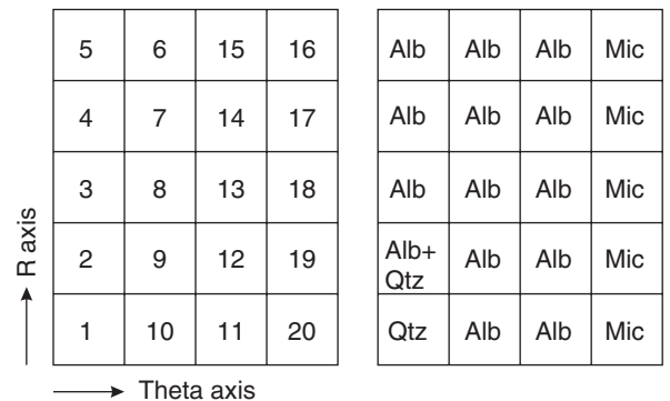
Fig. 15. A 5 \times 4 grid in 0.1 mm increments of the granite slab. The location of the data points is shown in the figure on the left. The mineral at each point is shown in the figure on the right. Mineral identification was performed solely by Raman spectroscopy. The minerals identified were quartz (Qtz), albite (Alb) and Microcline (Mic).
