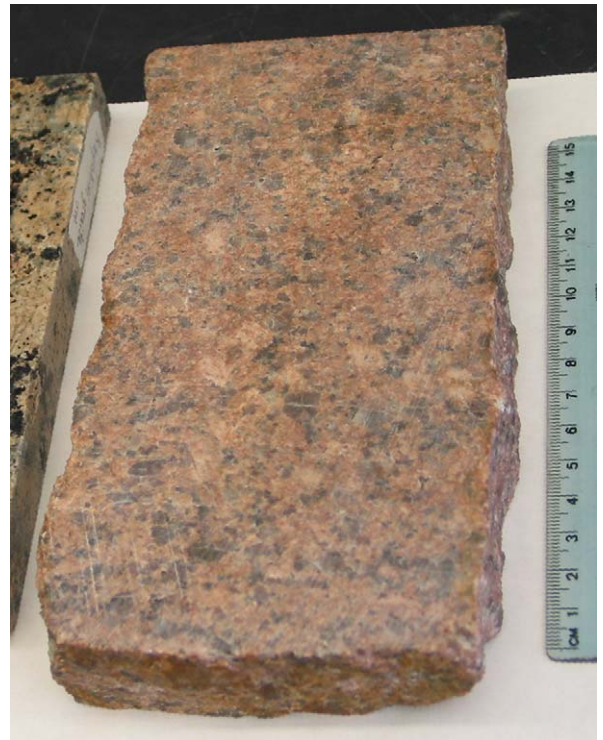
Fig. 14. A slab of Rapakivi granite (from J. Pasteris, Washington University) carried to the seafloor for DORISS/PUP testing.
