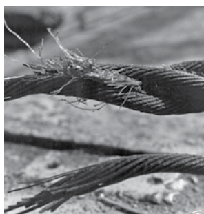
Steel support cables holding Alvin snap at the beginning of a dive. The pilot and observers scramble to safety, but Alvin sinks 5,000 feet to the seafloor.
