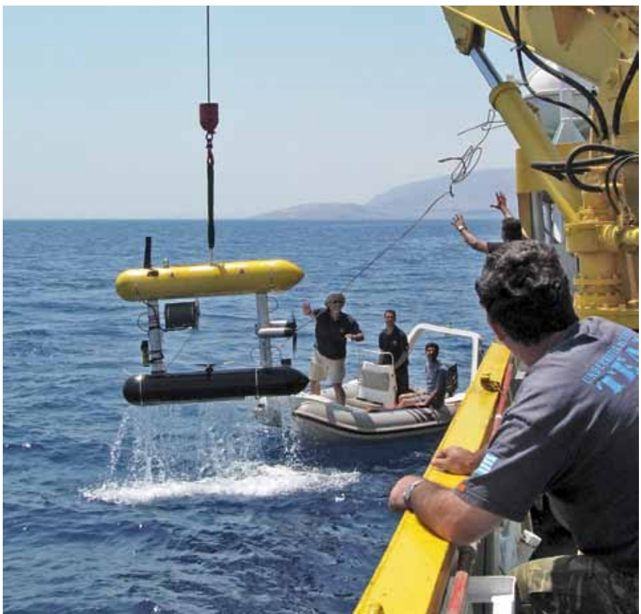
In 2005, a deep-diving WHOI autonomous underwater vehicle called SeaBED was used to survey and systematically photograph a shipwreck from about 350 B.C. off the isle of Chios.
