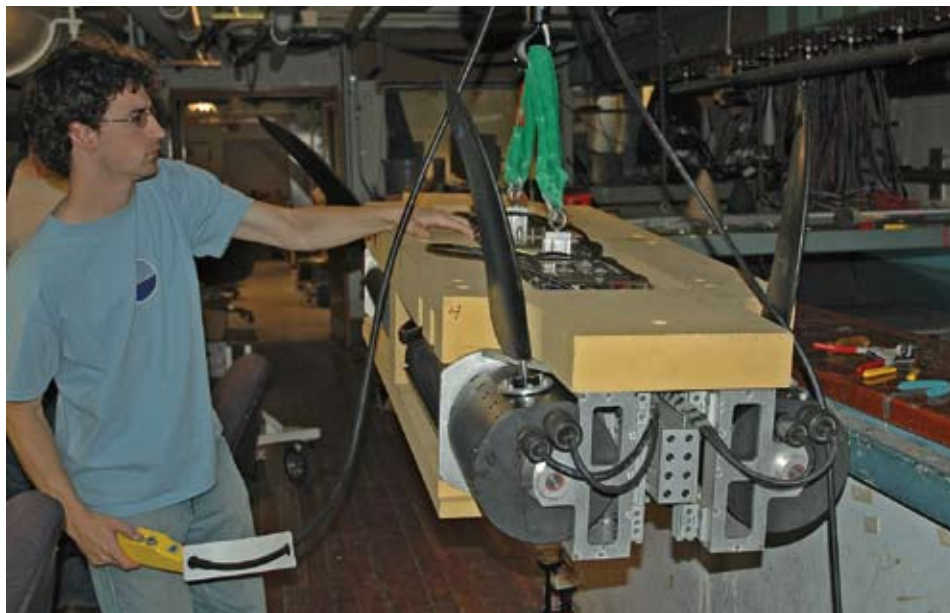
As an MIT/WHOI graduate student, Stephen Licht built an underwater vehicle called Finnegan (seen here without its yellow outside "skin") with flapping foils to enhance its maneuverability.
