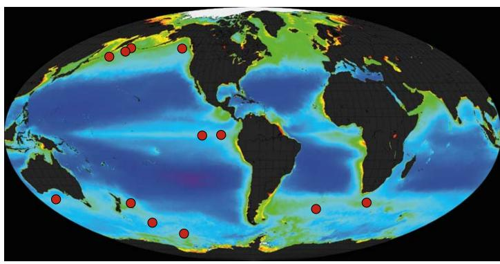
TESTING THE WATERS—Twelve small-scale experiments over the past decade in several ocean locations (red dots) consistently showed that intentional iron additions do result in phytoplankton blooms that help draw down carbon dioxide from the air. But the experiments have not determined how much carbon is transferred and sequestered in the deep sea, rather than quickly recycled back to the atmosphere.
