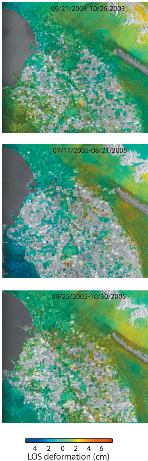
Figure 8. Phase (color) and amplitude (intensity) for typical interferograms in the Imperial Valley, spanning three different time intervals during the same time of year as the Obsidian Buttes swarm. Color scale is the same as in Figure 6.
