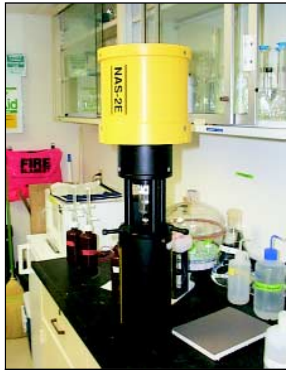
In situ nutrient analysers will increasingly be used for monitoring nutrient loading. Upon laboratory calibration, they can be deployed for periods of weeks to months. Photo by M. Trice.
