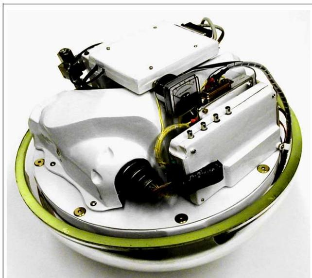
**Figure 1.** NEREUS MS with upper glass-pressure hemisphere removed.
