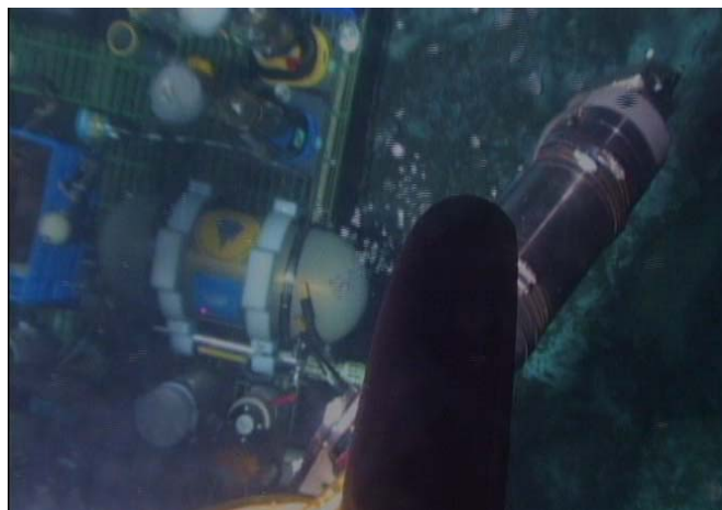
Fig. 5. Photo of TETHYS mass spectrometer (5,000 meter rated unit) operating during DSV Alvin dive mission off the coast of Southern California. The TETHYS instrument is mounted to the starboard side of the forward science basket. Small bubbles of free gas can be seen between TETHYS and the starboard manipulator arm.
