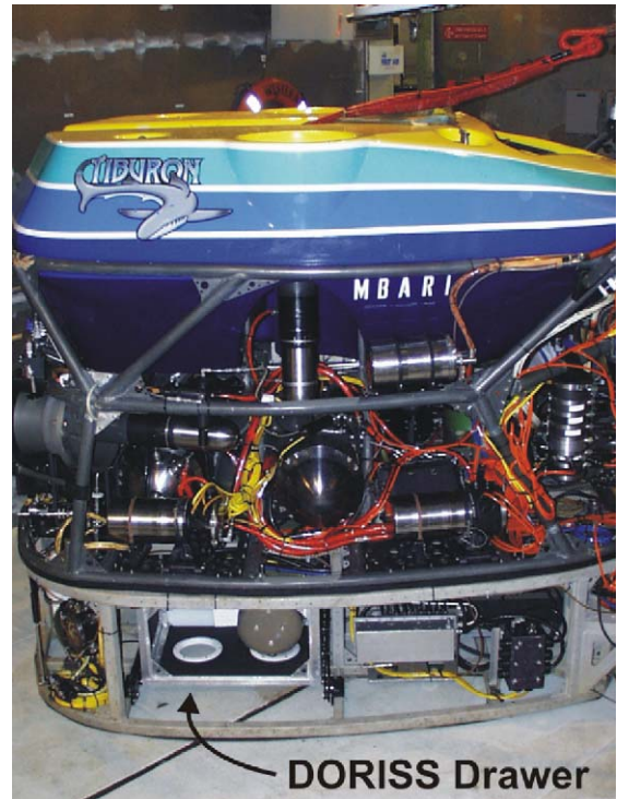
Fig. 1. MBARI's remotely operated vehicle "Tiburon", in side view. The base vehicle weight is 3084 kg. Front, with manipulators and cameras not shown, is to the right of the image. The syntactic foam pack that provides buoyancy is on top, the core vehicle power, thrust, telemetry, and computing, systems are housed in the middle. Below is the tool sled with the drawer used to house the DORISS system seen at bottom left.
