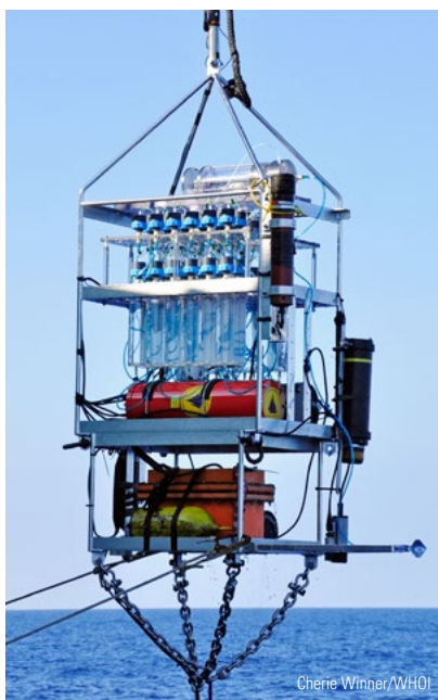
The fragile-looking Microbial Sampler-SID has collected and preserved deep-sea organisms never seen before.
