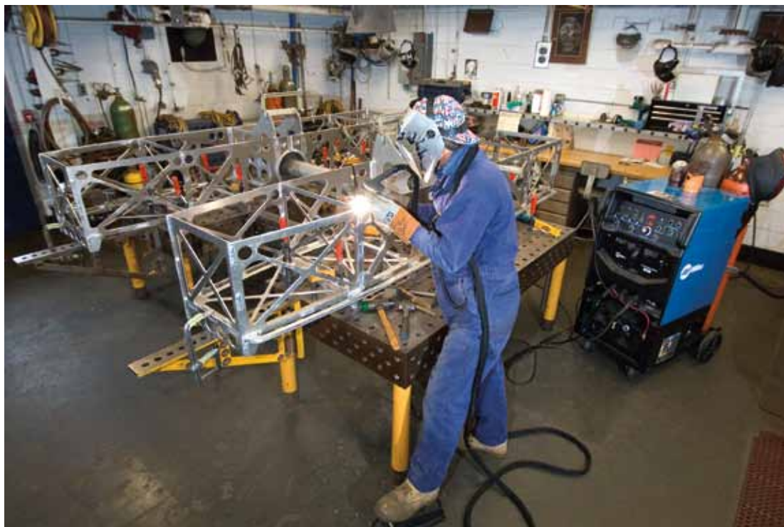
Geoffrey Ekblaw, lead welder in the WHOI mechanical shop, works on part of Nereus ' frame.
