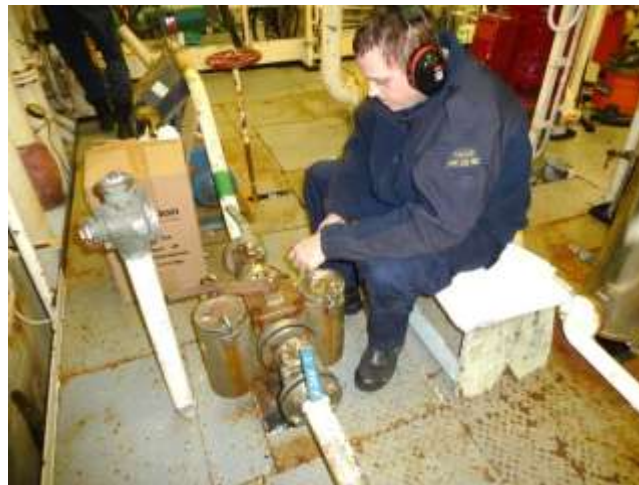
Figure 6. Seawater passes through a filter before going to the pump (in background). When the ship is in sea-ice the flow is switched from one filter to the other to allow the necessary frequent clearing out of slush from the filter.
