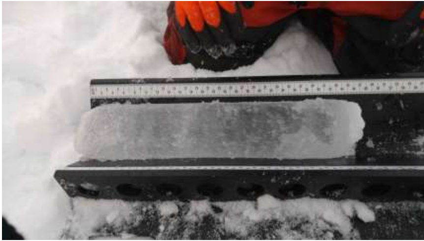
Ice Station 1, Site 1 Core A, Temperature/Salinity Core Top was very rough, bottom was a bit chipped.
