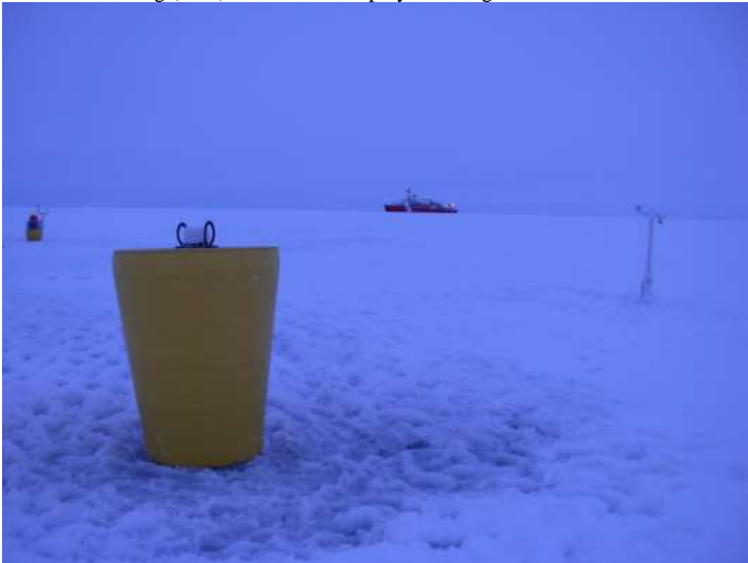
IBO 1 deployed on September 29, 2016 consisting of AOFB 34 (left), ITP 98 (center) and SIMB (right) shortly after deployment, with the CCGS Louis S. St. Laurent in the background.
