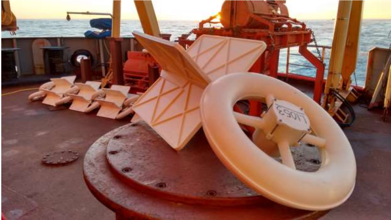
Figure 12 CARTHE drifters with floating element and wings connected by a flexible neck.
