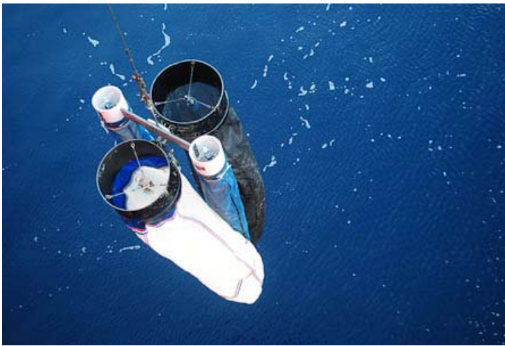
Figure 11. The 4-net 'Bongo' used on the JOIS program. Photo by Alex Kain.
