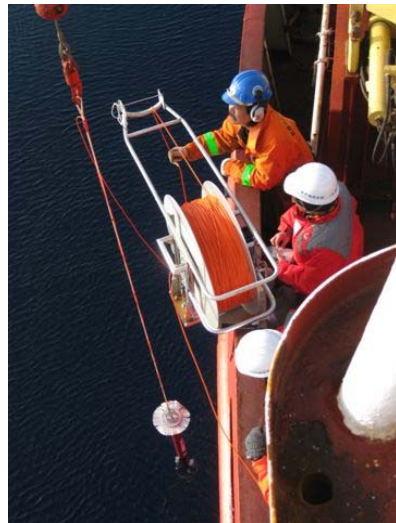
Figure 13. The winch and cable for the Turbomap
