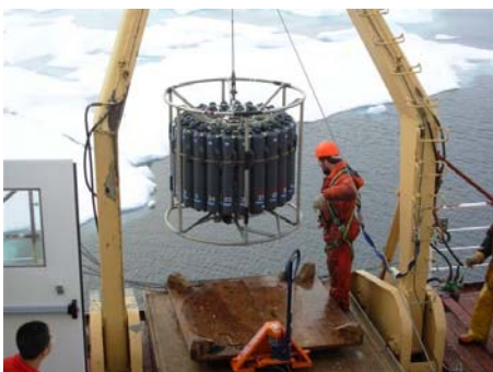
Figure 3. The 24-bottle rosette with the SBE9+ CTD is deployed by Mike Dempsey.
