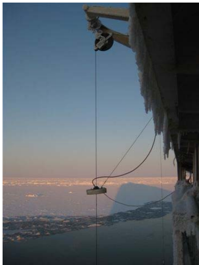
Figure 6. The 'de-icer' attached to the CTD wire.
