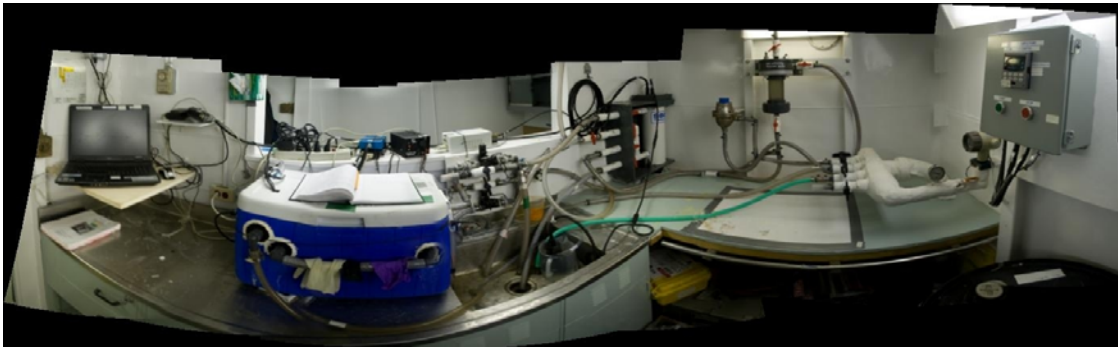
Figure 23. Seawater loop Lab including the Pump control, manifold, debubbler, flow control, TSG, COM and fluorometer in sink, blue cooler, and acquisition computer.
