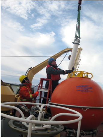
Figure 13. Installing the Upward Looking Sonar (photo Gertie Ward, acknowledgement to ARCUS PolarTREC)
